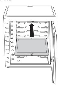
2 Plug the USB end of the dock connector cable into the USB port on the Charge and Sync Cabinet.
