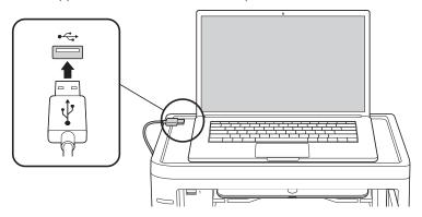
2 Connect the other end of the USB cable to the USB port  $\mathcal O$  on the back of the Charge and Sync Cabinet.
