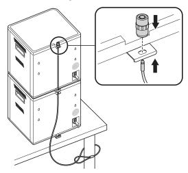
**NOTE:** Up to two Charge and Sync Cabinets can be stacked together.
