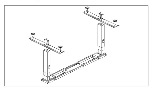
**Step 4**Install the two side brackets with Screws 4 pcs M6x12,
